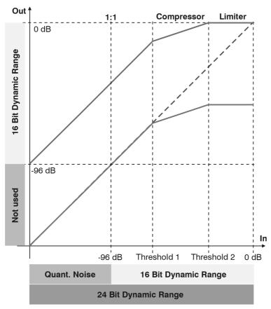
A look at the level relations during compression quickly reveals the necessity for 24bit recordings. If a signal remains unprocessed (straight broken line), the 16 bits of a signal are projected in CD format (x-axis) or the upper 16 bits of a 24-bit signal are projected onto the 16 bits of the CD format (y-axis). The lower bits of the 24-bit signal do not offer any advantage, since they are projected onto a range below -96 dB, which is not utilized by the CD.
