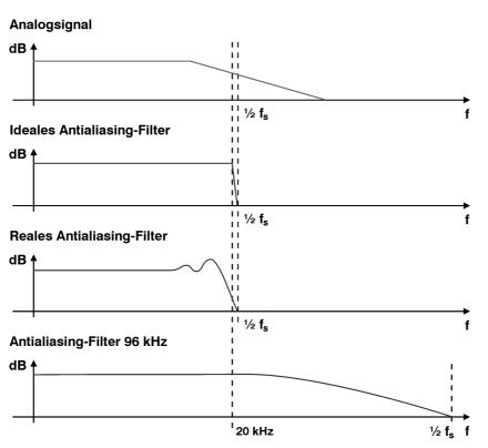
While the frequency spectrum of a natural audio signal falls off towards the high frequencies, it generally contains components that lie above the half sampling sampling rate. To remove them, a steep edge filter is required, which does not affect the audio signal. Real filters, however, show a less steep filter edge as well as ripple in the transition region. With doubled sampling frequency, the problem is disappears since the edges are very flat and the filter can be constructed much simpler.
